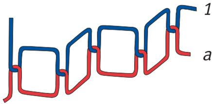
For elastic joining, closing and decorative seams (e.g. attaching rubber band to edge or sleeves) zig-zag double lockstitch is used
