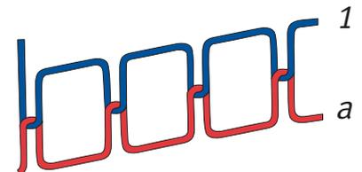
For joining and closing seams (e.g. closing of bra cup) double lockstitch is used
