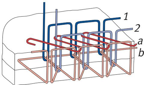
For flat seams and hems (e.g. elasticated leg seam)
