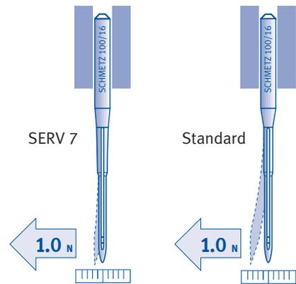
The SERV 7 needle's optimized humpscarf also prevents skip stitches which easily occur when sewing elastic materials and multiple layers. The humpscarf ensures that even when the loop is small or missing, there is sufficient space between the bottom of scarf and the needle thread. The looper or hook point can catch the needle thread securely every time.
