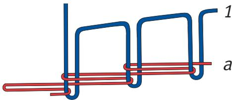
For elastic closing seams (e.g. joining of side pieces)
